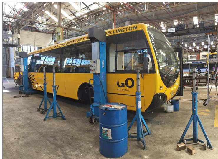
Right: Moving ahead to 20 December 2017, despite the trolleybuses now having all been withdrawn, 361 was still waiting for its conversion. On this date it was jacked up and missing its front axle.
