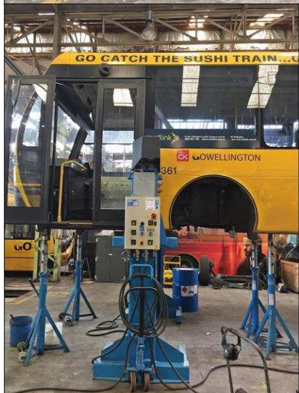
Right: Moving ahead to 20 December 2017, despite the trolleybuses now having all been withdrawn, 361 was still waiting for its conversion. On this date it was jacked up and missing its front axle.
