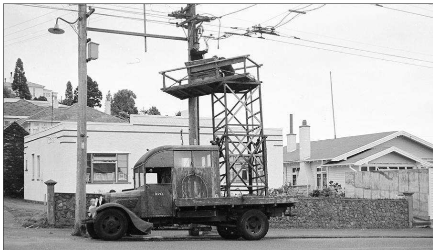
This ancient-looking tower wagon was probably the sole maintenance vehicle helping keep New Plymouth's four trolleybuses running. Maybe a keen-eyed reader from the area is able to offer some more information as to the make of this vehicle and maybe even where it was photographed. The NP system closed fifty-three years ago on 7 October 1967. Photo: Graeme Bennett.
