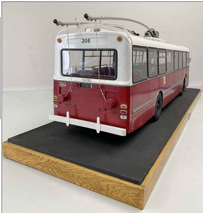
VOLVO B58 TROLLEY BUS CHASSIS ELECTRICAL EQUIPMENT: BROWN BOVERI MOTOR: 1756HP. CONTROLLER: THYRISTOR CHOPPER WITH TELMAR CURRENT RETARDER 68 CHASSIS SUPPLIED TO WELLINGTON CITY TRANSPORT: 1981-86
